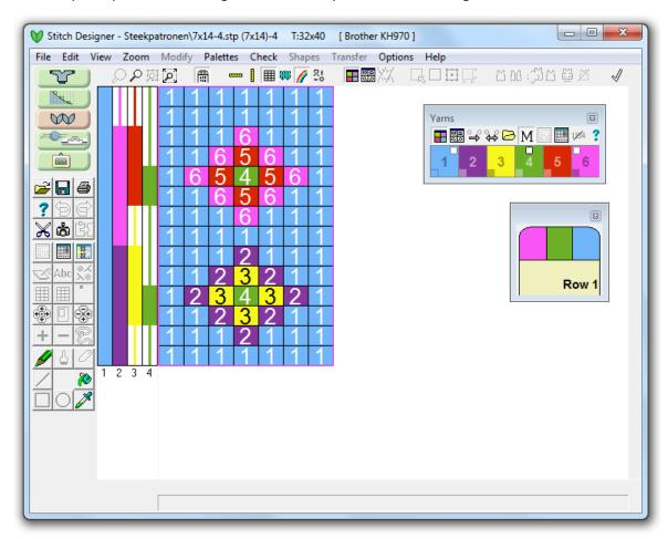
The Yarn numbers / Feeders setting determines the order in which the colors will be knitted. This setting is used by the CB-2 software when knitting a 4 color fairisle rib jacquard. In DesignaKnit this setting is called Jacquard, Color Separation B.
