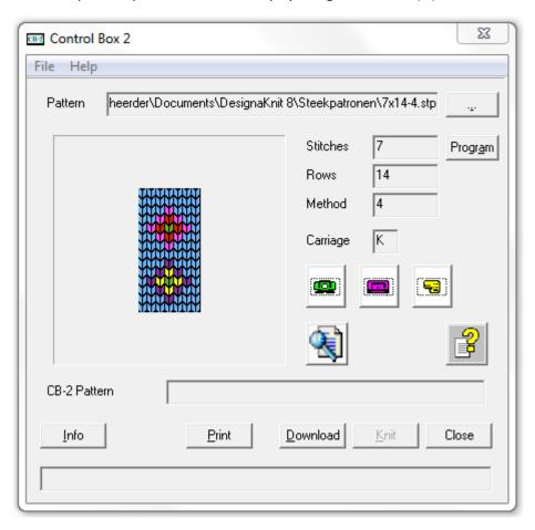
The stich pattern 7x14-4.stp has maximum 4 colors in a row which results in Method 4. The total number of colors used in the stitch pattern is 6, which means that the stitch pattern can be knitted with the KRC1000E, KRC1100M or EC-2000 color changer without the need of rethreading.
